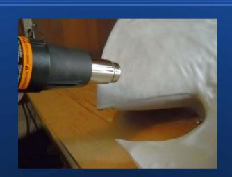
•Clip both front pieces to the form & flip the form on it's front. Wipe the inside shoulder & the curved edge of the back piece with cleaner to remove the oil and insure a good bond. Place the back piece over the form and use the heat gun & pressure to join the pieces. Their should be a lot of overlap at the shoulder this helps to keep the collar more stable. At the top of the neck where you curved over the ½ inch this should wrap over the front piece.
