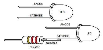
Typical resistor values are a few hundred ohms. For a two hundred twenty ohm resistor (which is a good value for most LEDs) the three color stripes (seen in the diagram) are red, red and brown.
